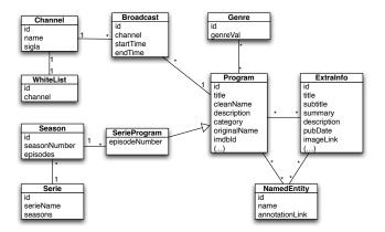
Fig. 4. The EPG+ Data Model
