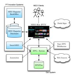
Fig. 2. Integration of EPG+ with PT Innovation systems
